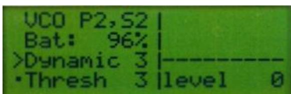
In this mode the display shows "**VCO**". Constantly shown are the level of signal in graphical and digital appearance, the capacity of the accumulator, chosen power, the sensitivity, the level of co – working of the sound and the working mode, as follows:
